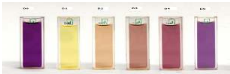
Fig. 2 - Consumption of methanolic solution of DPPH radical by colour change (from purple to yellow) in the five dilution (D 1 , D 2 , D 3 , D 4 and D 5 ) compared to the control D 0
